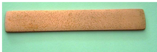
Figure 3. Pitting corrosion on a copper strip
